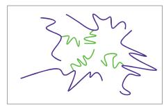
Rubber side chains cluster together inside the adhesive layer and "hide" the rubber properties inside the acrylic backbone. Adhesive appears like an acrylic and is easy to die-cut.
