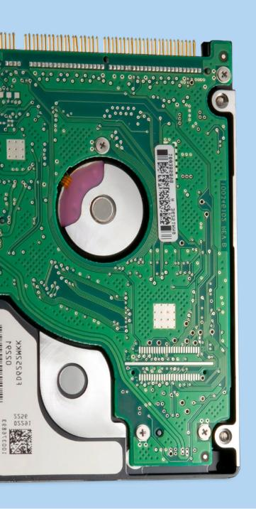
Printed Circuit Boards (PCBs) are used to hold and connect electronic components and are found inside every electronic device. They are assembled in an automated process, where they are exposed to extreme heat and chemicals. During assembly, traceability of the PCB is vital – and this requires the use of identification and tracking labels.
